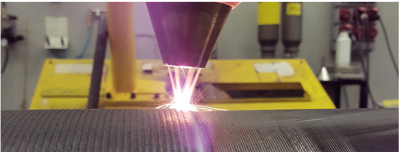
Laser coating with a laser welder
